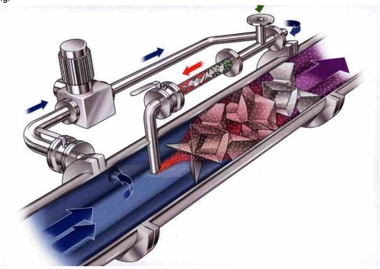
The DN 700 main contactor mixers each oxygenate between 500 to 1500 m3/hr of water and each feed four filters. There is no requirement for downstream reactor vessels or towers with all gas dissolving being carried out in line.
